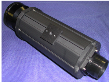
Figure 1 – Mounting bracket on Thermal-Eye TSC4500
