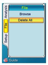
Press the M or ➤ Keys to enter the "File" menu. Press the ▼ Key to highlight and select "Delete All", then press the M or OK Keys. When the dialog box is displayed, press the OK Key to to delete all files or C Key to cancel the operation.
