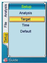
Press the **M** or **OK Key** to enter the "Target Setup" option.
