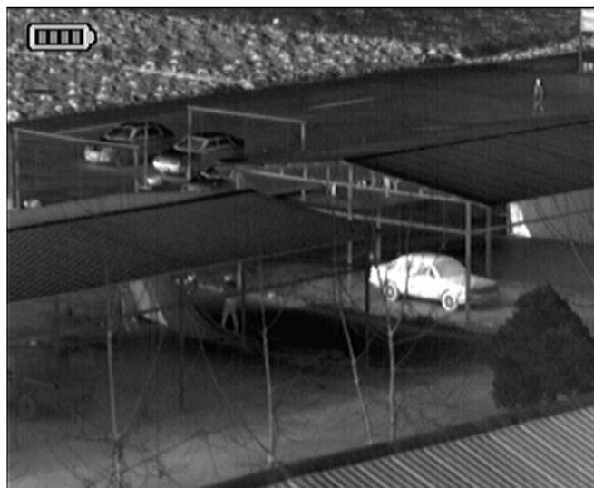
The system continuously monitors the power supply voltage. If the power is not enough, there will be an icon to warn the user, if user does not turn off the SPOTTER-T14X, the system will automatically shut down after a minimum voltage level is reached.
